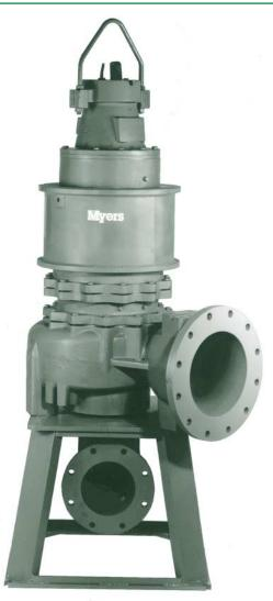
THE 12VLDP AND 12VLXDP (EXPLOSION-PROOF) SUBMERSIBLE DRY PIT WASTEWATER PUMPS ARE DESIGNED ESPECIALLY FOR HIGH FLOW MEDIUM HEAD APPLICATIONS SUCH AS: large municipal stations, treatment plants, transfer stations and dewatering. The pump handles solids up to 5½ inches in diameter and 2 available motor speeds make it ideal for most high flow wastewater applications. Call your Myers distributor, or the Myers Ohio sales office at 419-289-1144 for more details.
